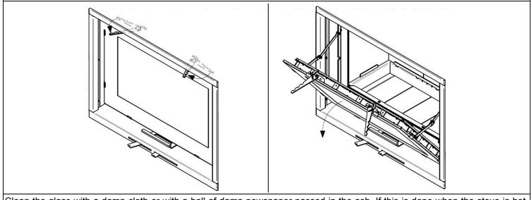
Clean the glass with a damp cloth or with a ball of damp newspaper passed in the ash. If this is done when the stove is hot, the glass could explode. Do not use aggressive or abrasive chemical products. Use newspaper with water and a little ash.
