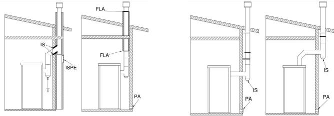
Key: IS - Insulator; ISPE - Inspection; T - T fitting; FLA - Hermetic closure flange; PA - External air intake
