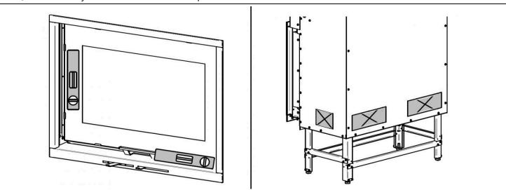
2. Proceed with the connection of the smoke duct and the flexible pipes for the convective air and then with the creation of the cladding.
