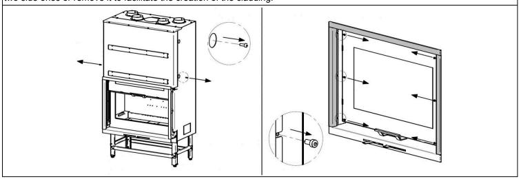
2. Using a spirit level, adjust the position of the monoblock with reference to the glass and the lower frame by adjusting the feet for this purpose. The internal part of the lower frame represents the level of the cladding. If the ventilation kit is NOT present, it is necessary to break the side and rear pre-cuts.
