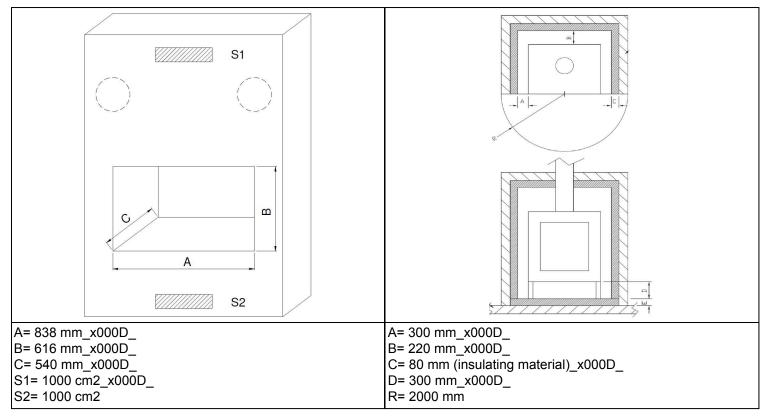
If you intend to install the product with a ventilation kit, you must take into account the possibility of accessing it for subsequent maintenance, which can however be carried out from inside the product. If the air passage sections described in the instruction manual are not guaranteed, anomalies in the correct functioning of the product may occur.
