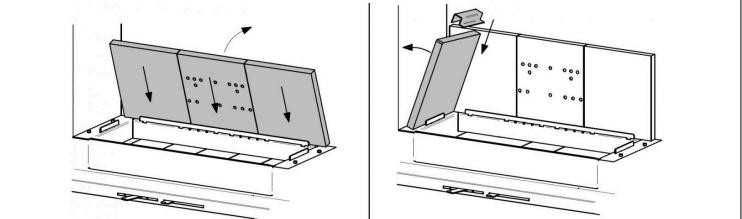
2. Pre-assemble the upper deflector with the two reinforcing "C"s and three vermiculites. Once positioned above the side brackets, push it towards the back.
