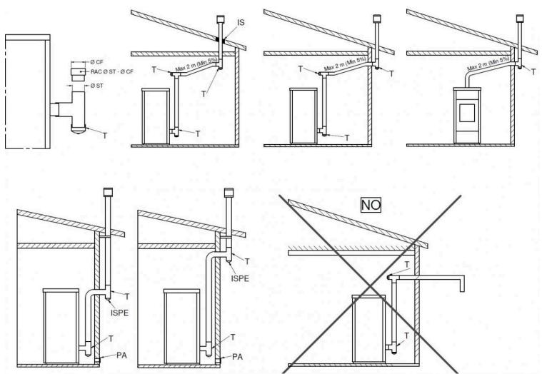
Key: T - T fitting; Ø ST - Stove diameter T; RAC Ø ST Ø CF - Stove and smoke duct connection; Ø CF - Smoke duct diameter; IS - Insulator; ISPE - Inspection; PA - External air intake
