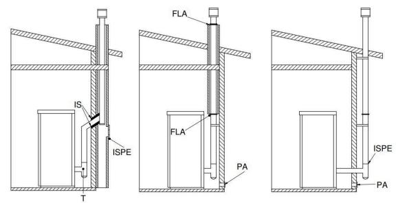
Key: IS - Insulator; ISPE - Inspection; T - T fitting; FLA - Hermetic closure flange; PA - External air intake
