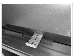
Secondary air adjustment device: 100% open in this position
