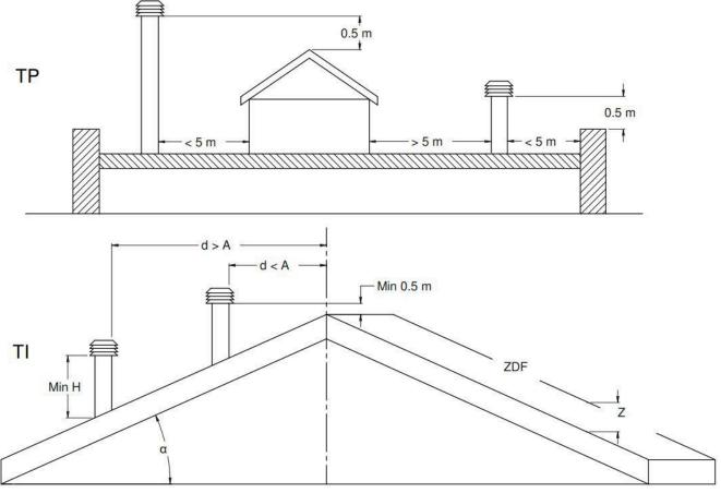
Key: TP - flat roof; TI - sloping roof; d - distance; ZDF - reflux zone
