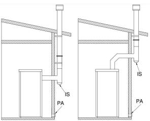
Key: IS - Insulator; ISPE - Inspection; T - T fitting; FLA - Hermetic closure flange; PA - External air intake
