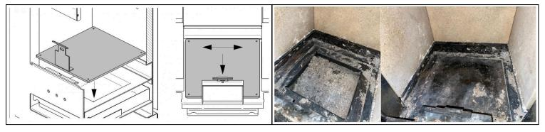
Vacuum the fire bed with an ash vacuum cleaner or remove the ash with a brush to ensure correct coupling. Suck up the ash that can get stuck in the front primary air slot or through the 3 front holes.
