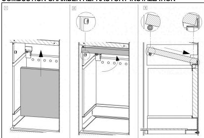
For the EVSL5 and EVSL6 install the upper vermiculite as follows:
