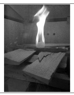
Do not add any more wood until the load has been consumed. Close the adjustment devices if the fire has ignited well. If the wood is damp or the flue does not have much draft, it is advisable to leave the door ajar. The moment you close it and the fire tends to go out, reopen the door and favor the complete ignition of the initial charge.
