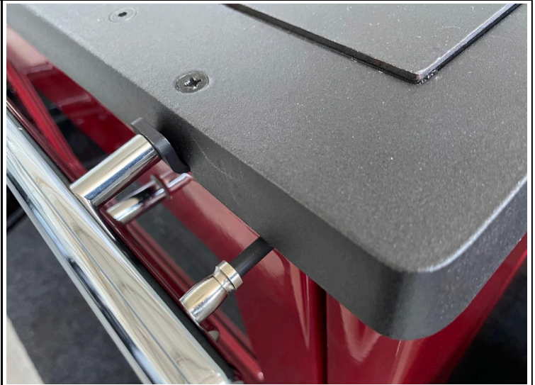
Fume outlet adjustment device: closed when the lever is pushed inside the stove. Open when the lever is pulled out.
