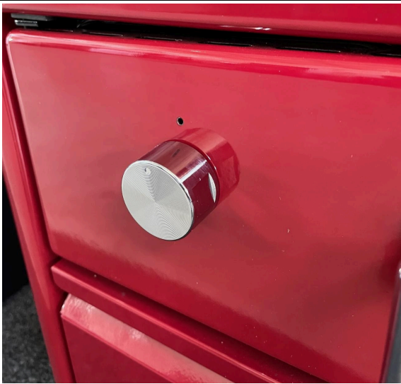
Primary air adjustment device. Closed in this position
