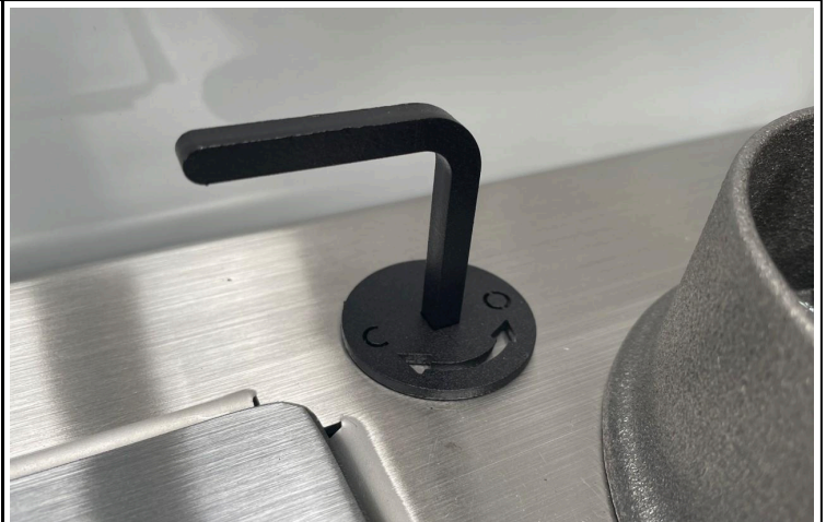
Smoke outlet register: turn the lever clockwise to open the register. Keep it closed during normal operation.
