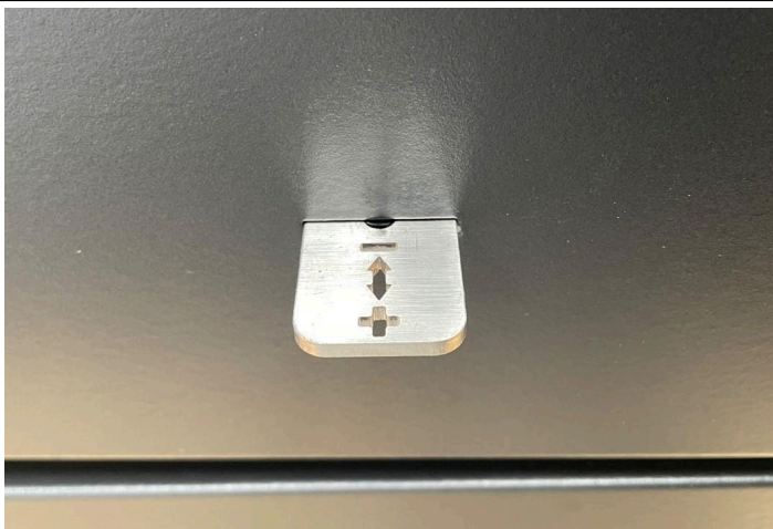
Primary and secondary air register. Open in this position. If pushed inwards the register is closed.
