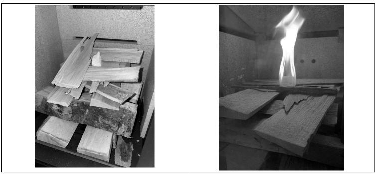
Do not add any more wood until the load has been consumed. Close the adjustment devices if the fire has ignited well. If the wood is damp or the flue does not have much draft, it is advisable to leave the door ajar. The moment you close it and the fire tends to go out, reopen the door and favor the complete ignition of the initial charge.
