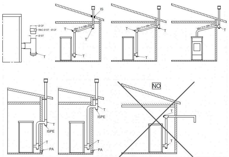
Key: T - T fitting; Ø ST - Stove diameter T; RAC Ø ST Ø CF - Stove and smoke duct connection; Ø CF - Smoke duct diameter; IS - Insulator; ISPE - Inspection; PA - External air intake
