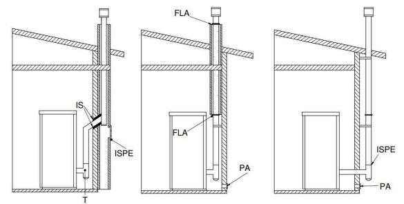
Key: IS - Insulator; ISPE - Inspection; T - T fitting; FLA - Hermetic closure flange; PA - External air intake
