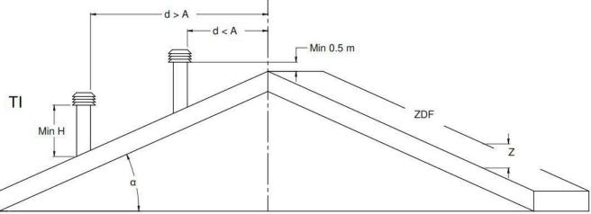
Key: TP - flat roof; TI - sloping roof; d - distance; ZDF - reflux zone
