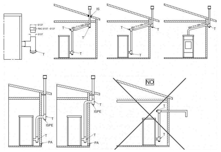
Key: T - T fitting;  $\emptyset$  ST - Stove diameter T; RAC  $\emptyset$  ST  $\emptyset$  CF - Stove and smoke duct connection;  $\emptyset$  CF - Smoke duct diameter; IS - Insulator; ISPE - Inspection; PA - External air intake
