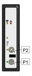
The remote control displays information regarding the operating status of the stove. A variety of data can be displayed and settings carried out according to the level of access by using the menu. Depending on the selected mode and on their position on the display, the data visualised may acquire different meanings.
